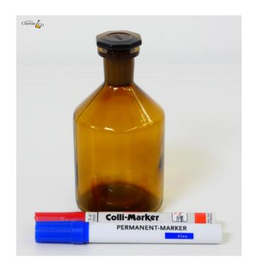
A lab bottle must be labeled with a permanent marker so that it is unambiguously clear what the content is.
